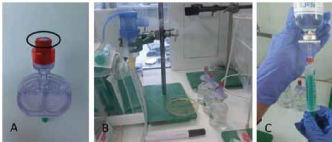
(A) Safeflow valve integrated in Mini-Spike® 2 Chemo V; (B) Experimental setup; (C) Withdrawal of NaCl after nebulisation
