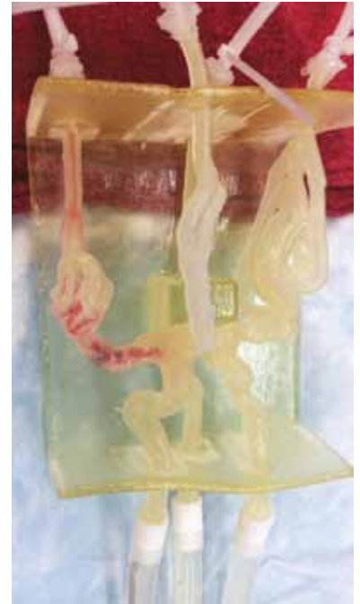
A 3D printed vascular phantom, with a manufactured blood clot to simulate a stroke.
