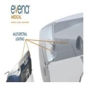
Evena's Wearable Eyes-OnTM Glasses Vascular Imaging System utilises Epson Moverio Smart Glasses technology platform to detect patient veins for precise IV placement
