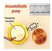
Bioengineers and scientists at Pennsylvania State University have developed an acoustofluidic pump that is powered by a piezoelectric transducer. The pump utilises the acoustic streaming effects generated by the oscillation of tilted sharp-edged structures that are hundreds of micrometres in length and that are constructed onto the sidewall of a microfluidic channel made of polydimtehylsiloxane (PDMS).
