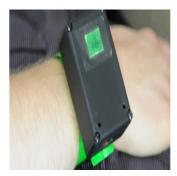
The coloured paper tags used to classify victims of mass casualty incidents may one day be replaced by plastic electronic wristbands capable of transmitting real-time data to emergency response control centres. The new tags are being developed by an international team of researchers at Fraunhofer-Institute fuer Angewandte Informationstechnik (FIT), as part of the European BRIDGE project.
