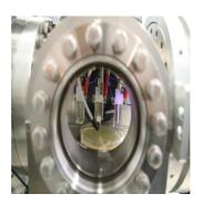
Plasma reactor: The RUB team generates atmospheric-pressure plasmas and tests which effects UV radiation and reactive particles have on bacterial cells and molecules. Copyright: RUB, Photo: Jan-Wilm Lackmann
