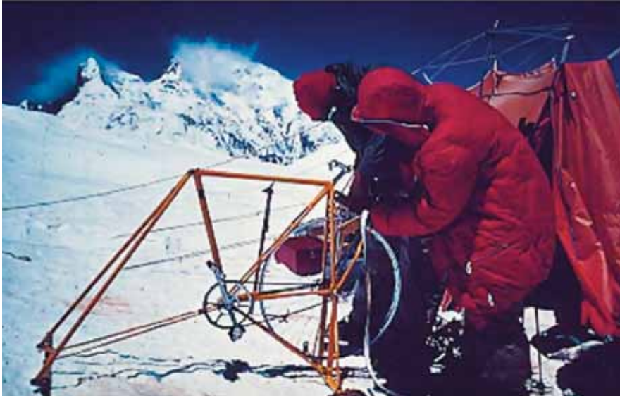
Michael Ward and John West assembling the stationary cycle to make measurements of maximal oxygen consumption at an altitude of 7440m (24,400 ft). These are the highest reported measurements to date.
